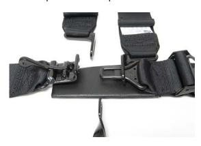
**3.** Slide the Anti-sub Strap Buckle over the male part of the Lap buckle.
